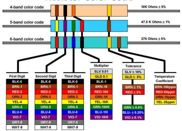
**Resistor Color Codes:** Resistors are devices that limit current flow and provide a voltage drop in electrical circuits. Because carbon resistors are physically small, they are color-coded to identify their resistance value in Ohms. The use of color bands on the body of a resistor is the most common system for indicating the value of a resistor. Color-coding is standardized by the Electronic Industries Association (EIA).
